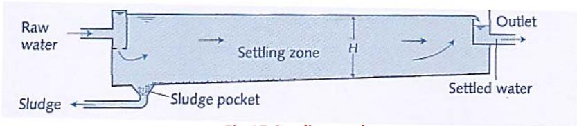
**Fig 15 Settling tank**
