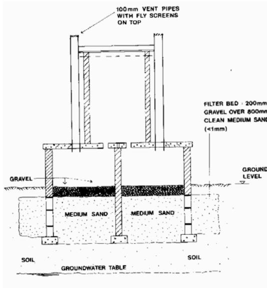
**Fig 36b Raised alternating twin-pit VIP latrine**
