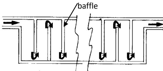
**Figure 14 Baffled-channel flocculators**
