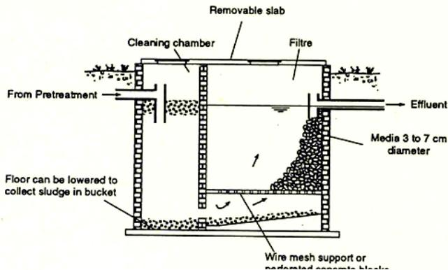
Fig 33: Anaerobic filter
