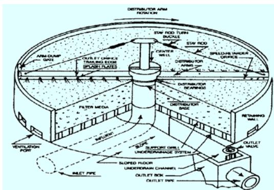
**Fig 24 Section of a trickling filter (EPA)**
