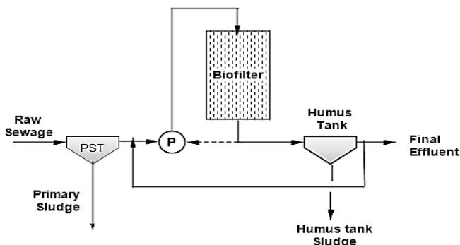
Fig 30a A Bio-tower filter systems
