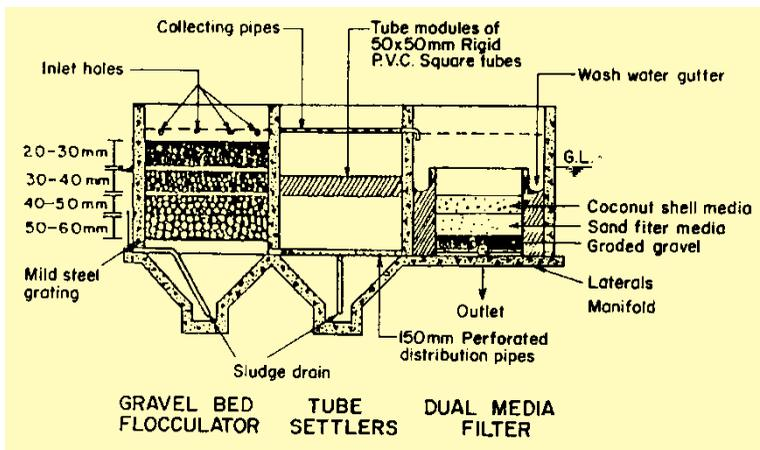
**Figure 17: Flow diagram of upflow-downflow Plant (Schulz & Okun, 1984)**
