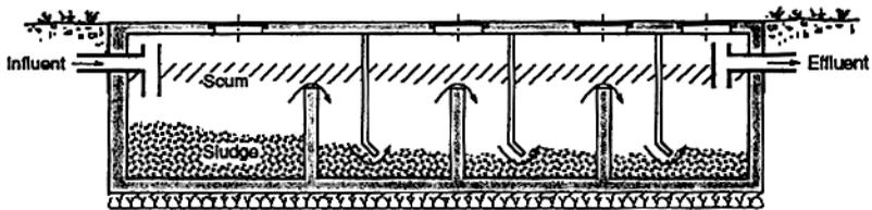
Fig 34: Baffled septic tank
