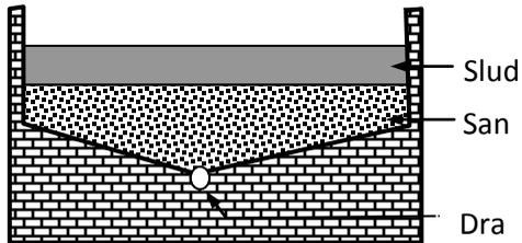
Fig 26: Sand drying bed
