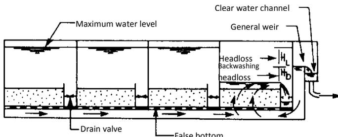
**Fig 16 Inter-filter-washing filtration units**
