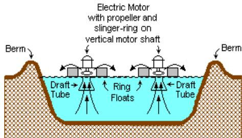
Fig 28: Completely mixed aerated pond
