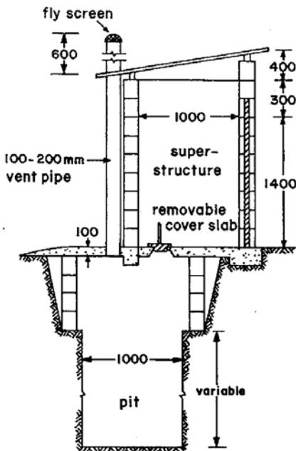
Fig 36a VIP cross section - dimensions in mm
