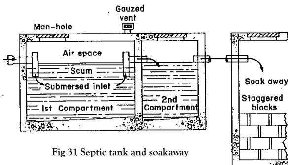
Fig 31 Septic tank and soakaway
