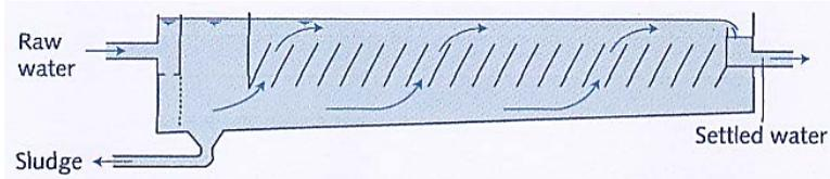
**Fig 15a Tilted plate settling tank**
