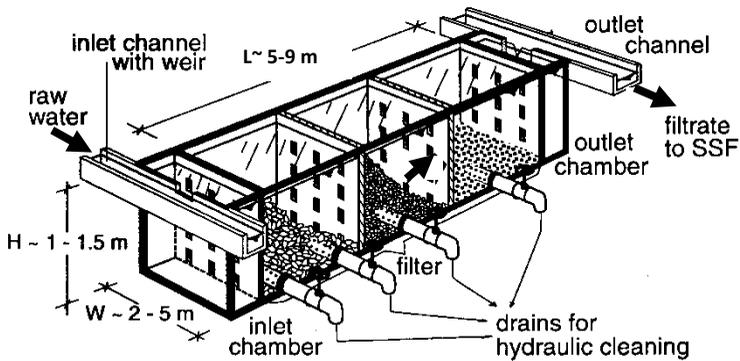
Figure 12: Horizontal flow roughing filter
