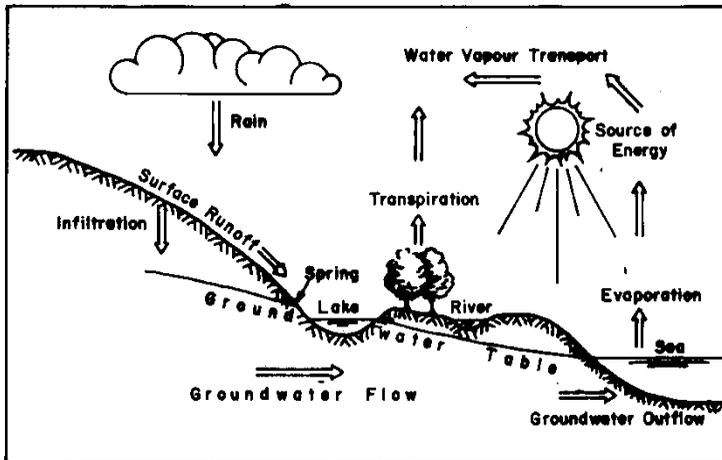
Fig 9 Hydrologic cycle
