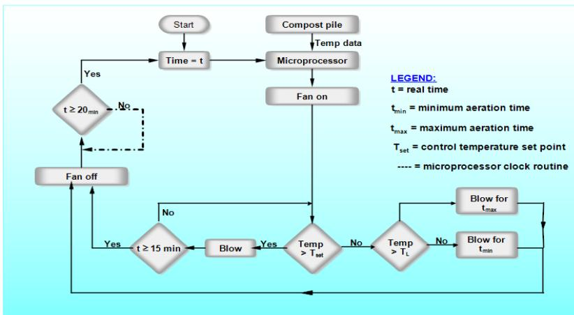
Fig 38: temperature control aerated composting pile
