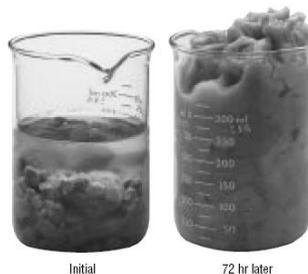
**Fig 4.6b Hydration of Imported Bentonite**
