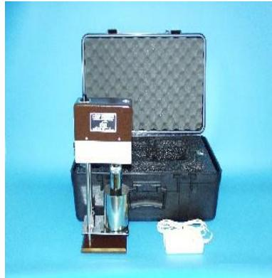
**Fig-2.3: Fann Viscometer**
