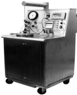
Fig 2.11a: HPHT Consistometer
