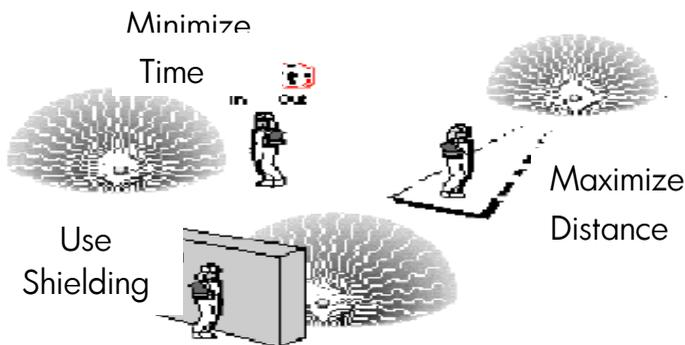
Figure 13: Illustration of Radiation Control
