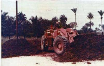
Fig 39c Front-end loader turning
