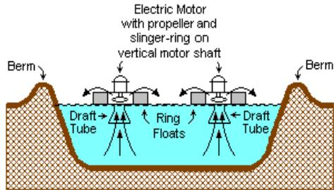
Fig 28: Completely mixed aerated pond
