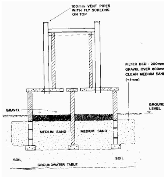
**Fig 36b Raised alternating twin-pit VIP latrine**
