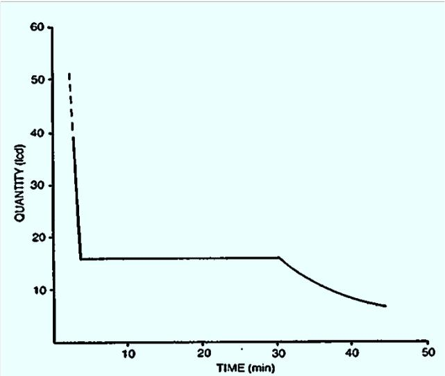
Figure 11 Graph relating domestic water consumption to collection time (Cairncross, 1987)
