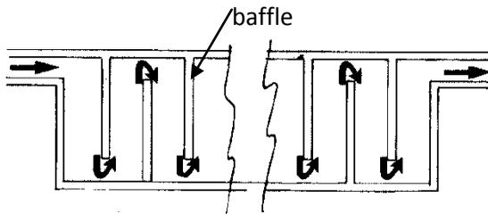
**Figure 14 Baffled-channel flocculators**
