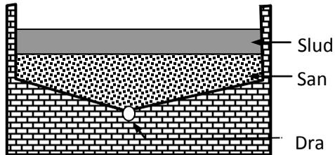
Fig 26: Sand drying bed
