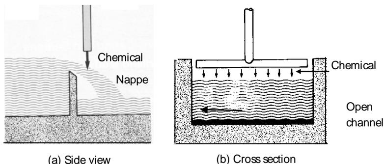
**Figure 13: A simple and reliable rapid mix system using sharp**
