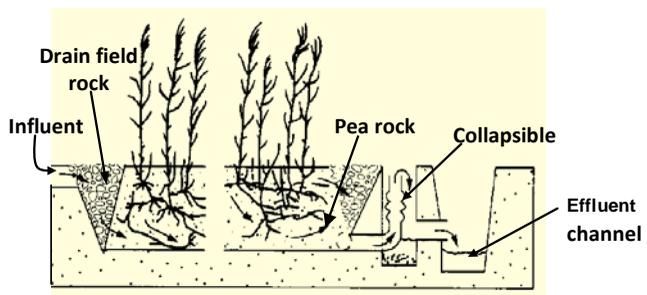
(SF), (Figures 35a and 35b), also called *free-water system*, and the *subsurface flow (SSF)* system (Figure 35c). Both of these are horizontal flow systems where wastewater enters at one end of a lined excavation and exits from the other end.
