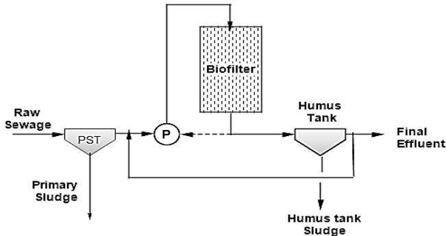
Fig 30a A Bio-tower filter systems
