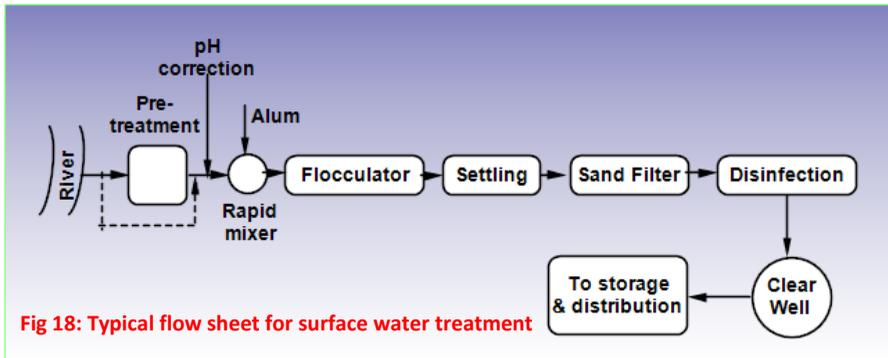
**Fig 18: Typical flow sheet for surface water treatment**
