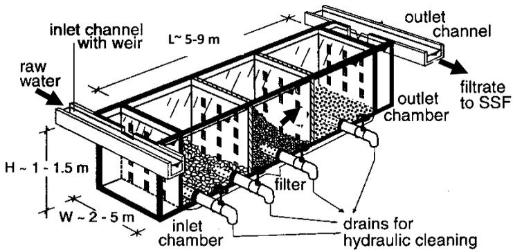
Figure 12: Horizontal flow roughing filter
