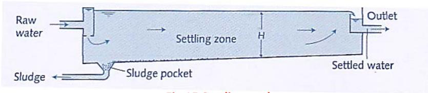
**Fig 15 Settling tank**
