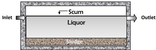
**Fig 32 Schematics of a Septic Tank**
