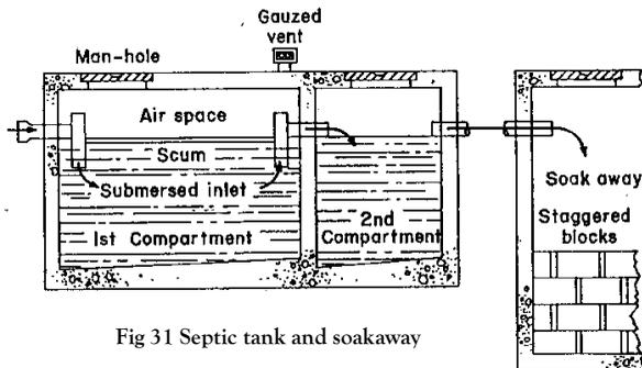
Fig 31 Septic tank and soakaway
