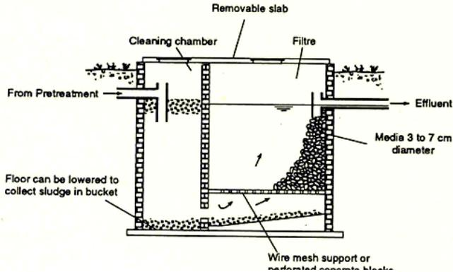
Fig 33: Anaerobic filter
