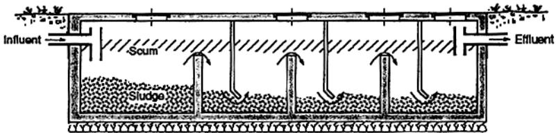
Fig 34: Baffled septic tank
