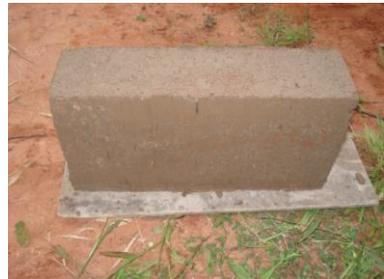
**Fig4.25d: Stabilized/solidified sample used for leachate and compressive strength tests.**
