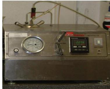
**Fig 2.14a: Autoclave system      Fig2.14b Ultra Sonic Cement analyzer**
