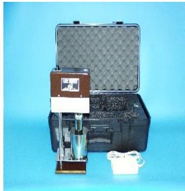
**Fig-2.3: Fann Viscometer**
