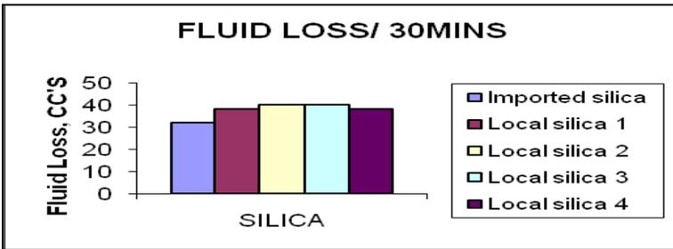
**Fig 4. 12: Fluid Loss per 30Minutes**
