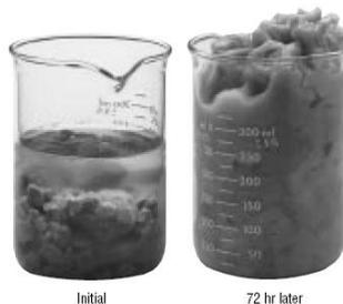
**Fig 4.6b Hydration of Imported Bentonite**
