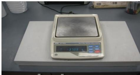
**Fig 2.9 Electronic Balance**
