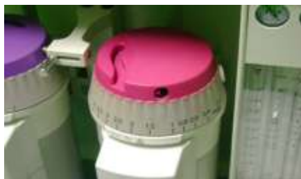
Fig 16: The Dräger Fabius Interlocking System
