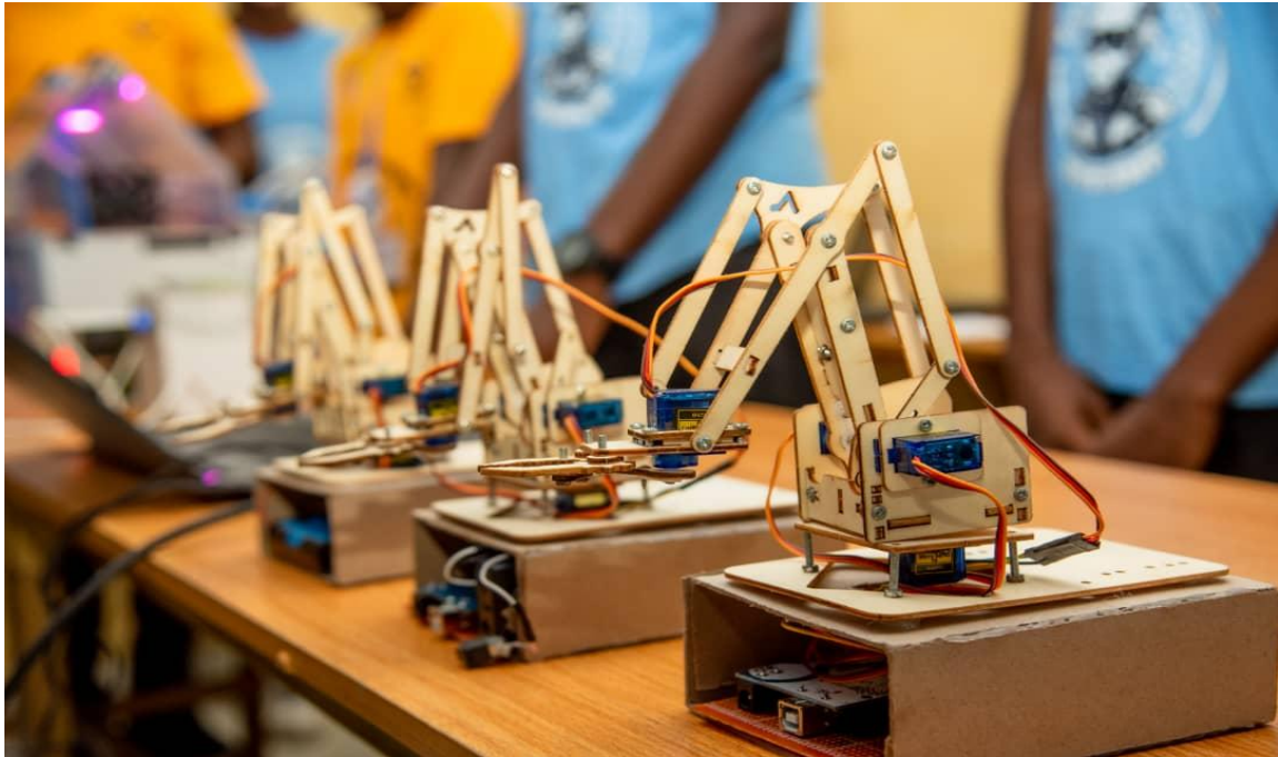
Plate 7 : Robotic Prototypes controlled via Bluetooth & GSM (CTY, 2024)
