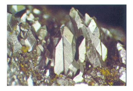
Figure 7. Galena (PbS): Typical habit and texture in host Limestone and Shales
