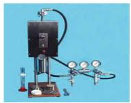
Fig-2.4: Low and HPHT Filtration cell
