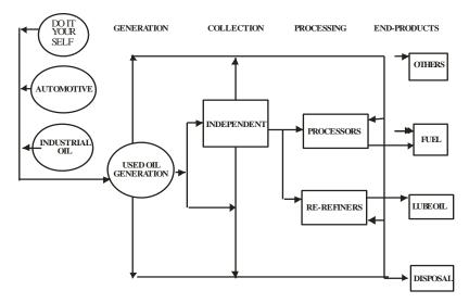
Fig 4.26: Proposed Used Lube Oil Management System in Nigeria:
