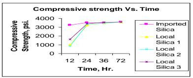
Fig 4.13: Compressive Strength versus Time
