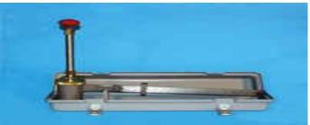
Fig-2.1: Pressurized mud balance
