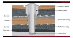
Fig.1-8: Casing types in cementing operations
