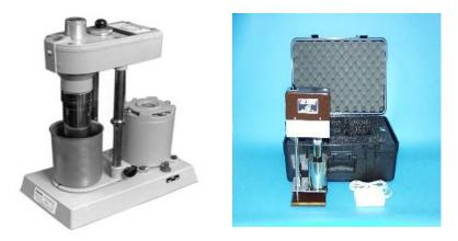
Fig-2.3: Fann Viscometer
