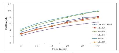
Fig 4.18: Fluid loss with time after aging at 80°F.
