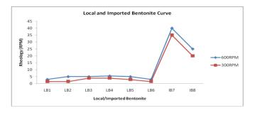
Fig 4.7: Local (LB1 - LB6) and Imported (IB7 - IB8) Bentonite Curve
