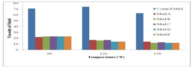
Fig 4.16: Viscosity of drilling fluids at different temperatures after aging (at 200rpm).
