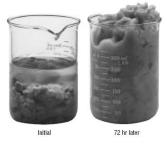
Fig 4.6a: Hydration of Local Bentonite
