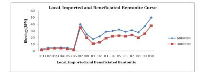
Fig4.8: Local (LB1–LB6), Imported (IB7–IB8) and Beneficiated (R1-R10) Bentonite Curve
