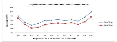
Fig 4.9: Imported (IB7 – IB8) and Beneficiated (R1 – R10) Bentonite Curve
