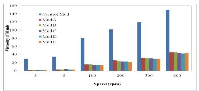
Fig 4.14: Viscosity of drilling fluids in (Cp) at different speed before aging at 80°F.
