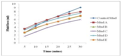
Fig 4.17: Fluid loss with time before aging at 80°F.
