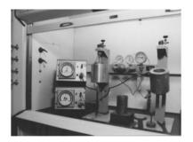
Fig 2.13: Static Fluid Loss Cell
