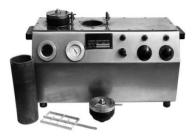
Fig 2.12: Atmospheric Consistometer
