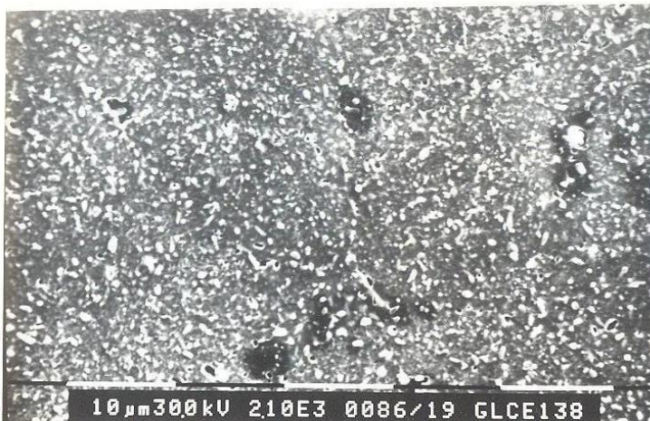
Fig. 10: Un-etched but polished surface of Alumina
