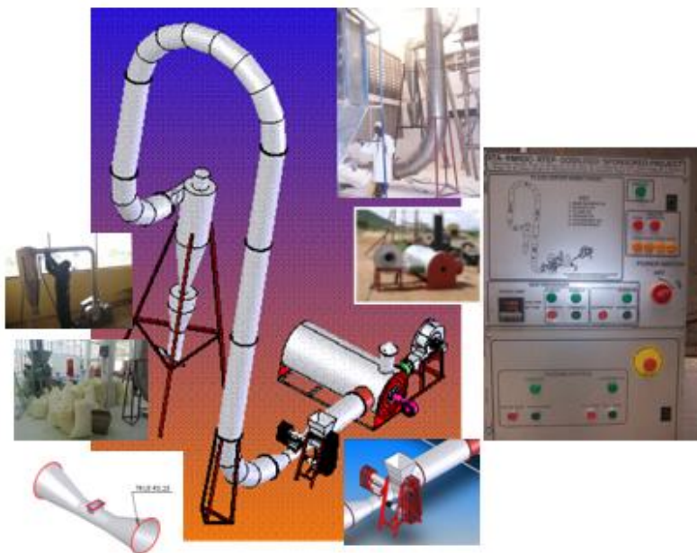
Fig 17: The flash dryer at different stages of fabrication
