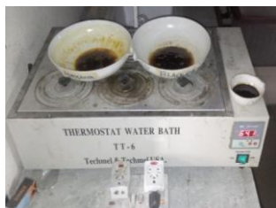
Figure I: Thermostat water bath used for the evaporation of liquid from extract.
