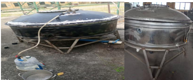
Plate 3: Mobile Biogas Digester with an improvised gas volume measuring device
